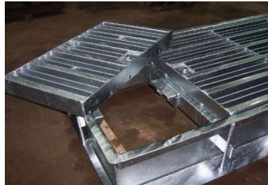
Standard Drainage Grid c/w special lift out section
